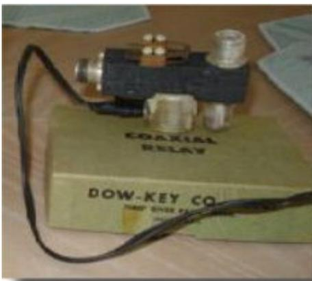
*Note: Dow Key Relay model DK60G2C 52 ohm 1000 Watts 115v to switch transmit and receive between the Valiant transmitter and Hammarland SP-600 receiver. This particular model has a separate set of contacts to mute the receiver. Click [here](#) for specifications.*
