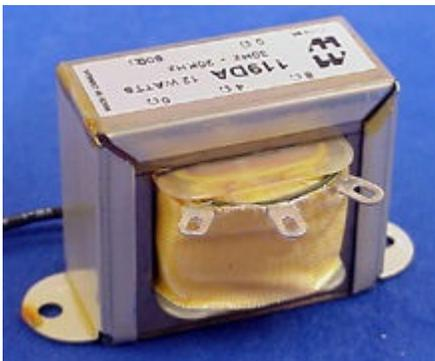
*Note: A Hammond Audio matching Transformer (Radio Daze part number HX119DA) was added to match the SP-600s 600 ohm audio output to an 8 ohm speaker. Here are the transformer's specifications:*
