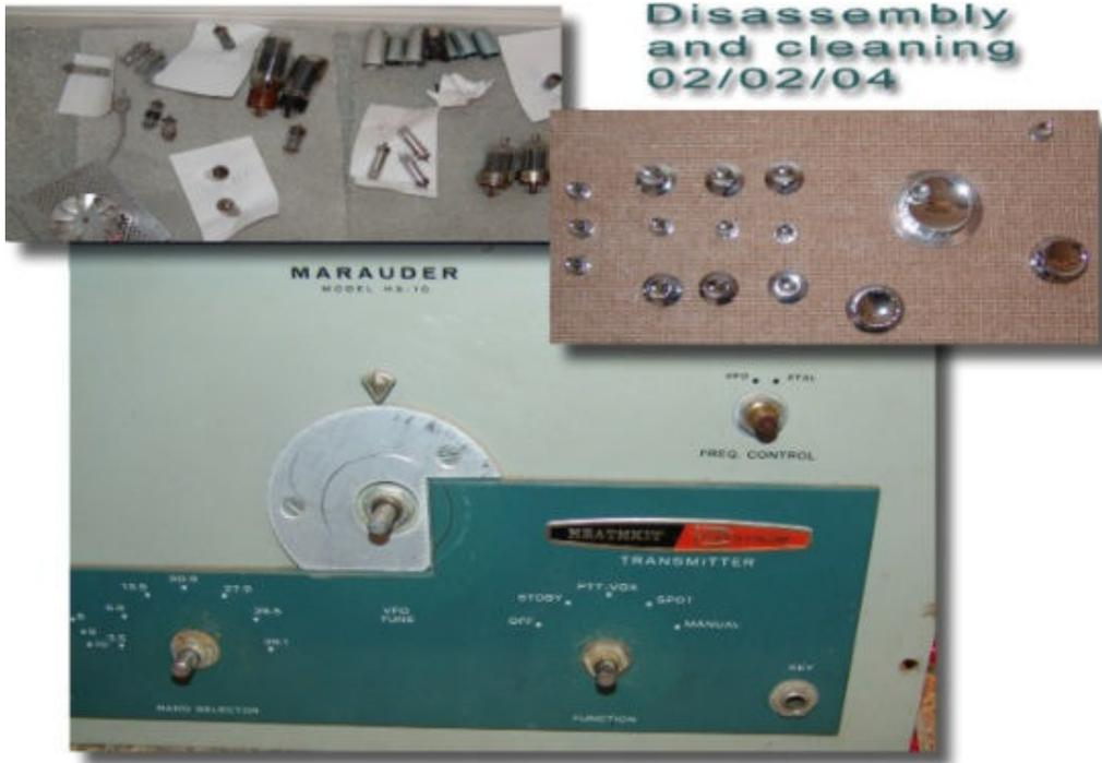
*Tubes and knobs have been cleaned and ready for reassembly. Front panel paint is in good shape and will only be cleaned.*
